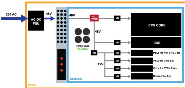
**Figure 4: Proposed server using 48V power delivery**
