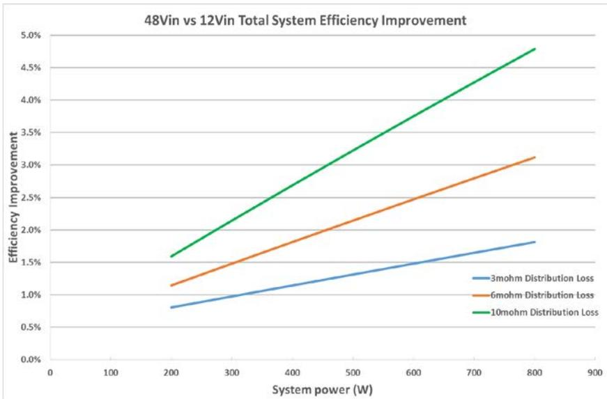
**Figure 5: 48Vin vs 12Vin total system efficiency improvement**
