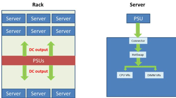
$$P_{\text{Distribution Loss}} = I^2 * R \text{ (distribution imped)}$$
