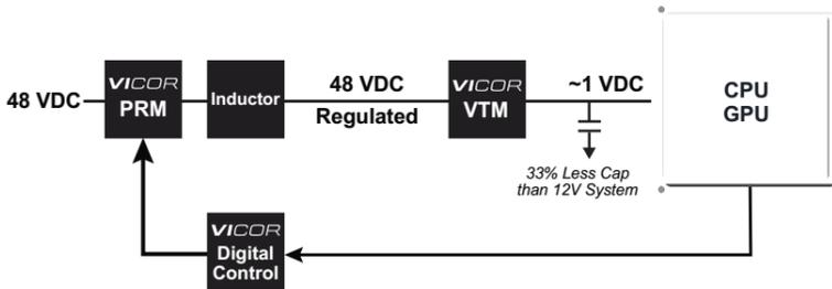
**Figure 3: 48V VR for processor/memory applications**
