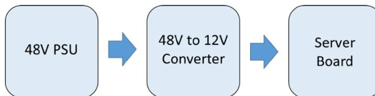
Figure 2: 48V-to-12V Two-Stage Power Conversion Architecture
