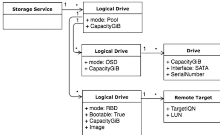
Figure 8. Data model for Ceph
