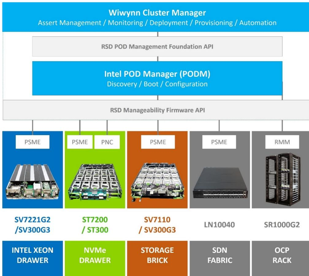
Figure 3. Architecture and building blocks of Wiwynn RSD solution
