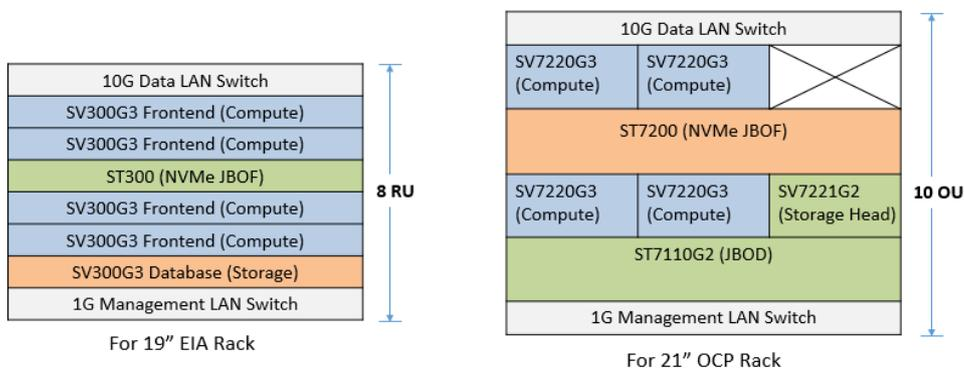
Figure12. Basic rack configuration for Wiyynn RSD POC
