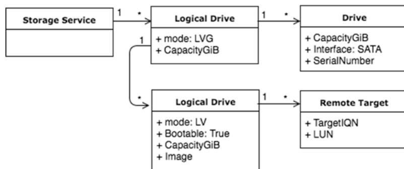
Figure 7. Data model designed for LVM
