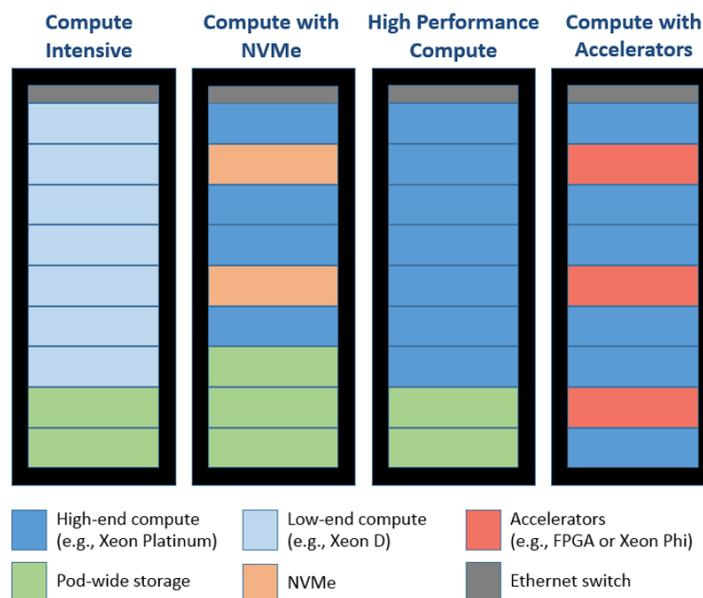
Figure 13. Example of Wiyynn® RSD Enabled pod
