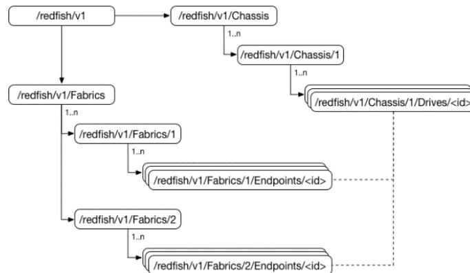
Figure 10. Redfish Schema to support the two-fabric ST300
