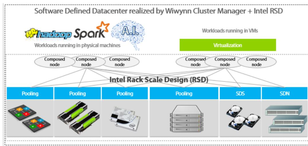
Figure 2. Intel® RSD, virtualization, and Cluster Manager realize complete SDDC
