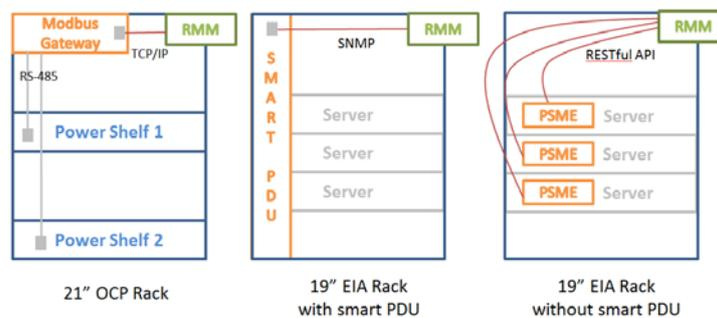
Figure 11. Flexible options of rack-level power consumption monitoring
