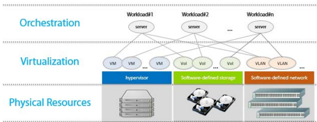
Figure 1. Virtualization deployed in datacenters today.
