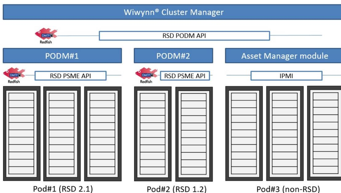
Figure 14. RSD and non-RSD pods coexist in a data center
