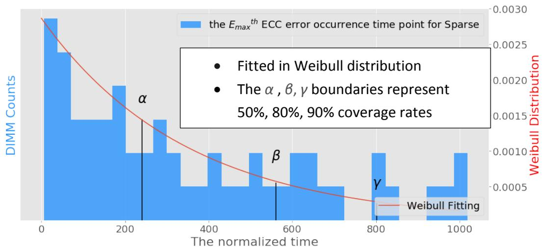
Figure 8 The  $E_{max}^{th}$  ECC error occurrence time point distribution for Sparse type
