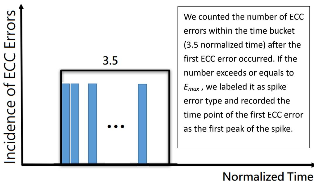
Figure 5: An illustration of the implementation of the error type labeling
