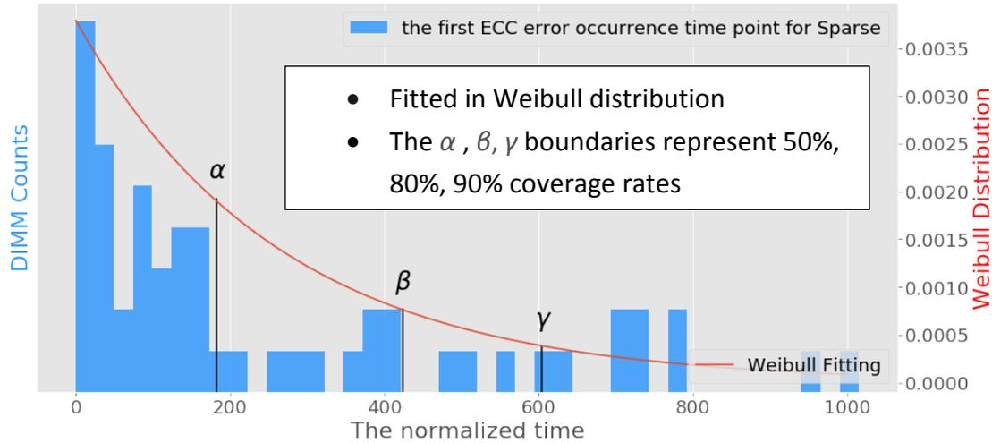
Figure 7: The first ECC error occurrence time point distribution for sparse type
