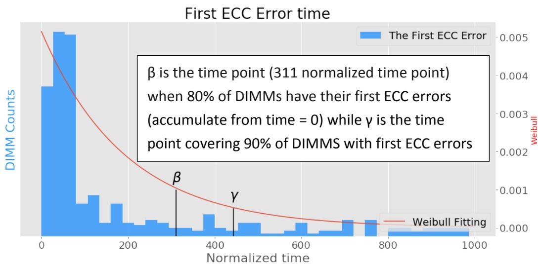
Figure 3: The Weibull distribution curve fitting on the ECC error distribution.
