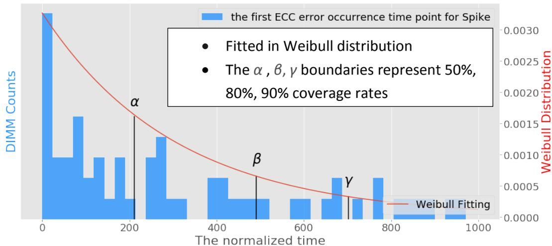
Figure 6: The distribution of the first ECC error occurrence time point for Spike type DIMMs
